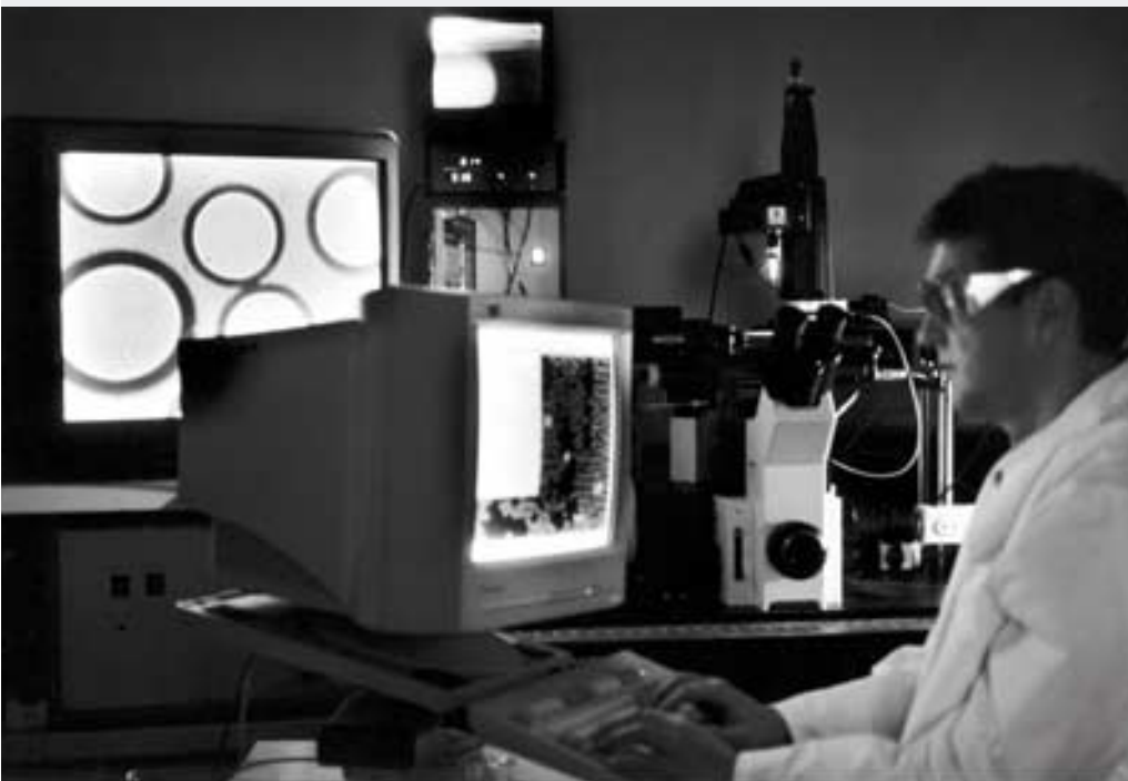
Fig. left: Andreas Fetsch at the PICKOscreen: a new type of device for screening substances on small polymer beads.
