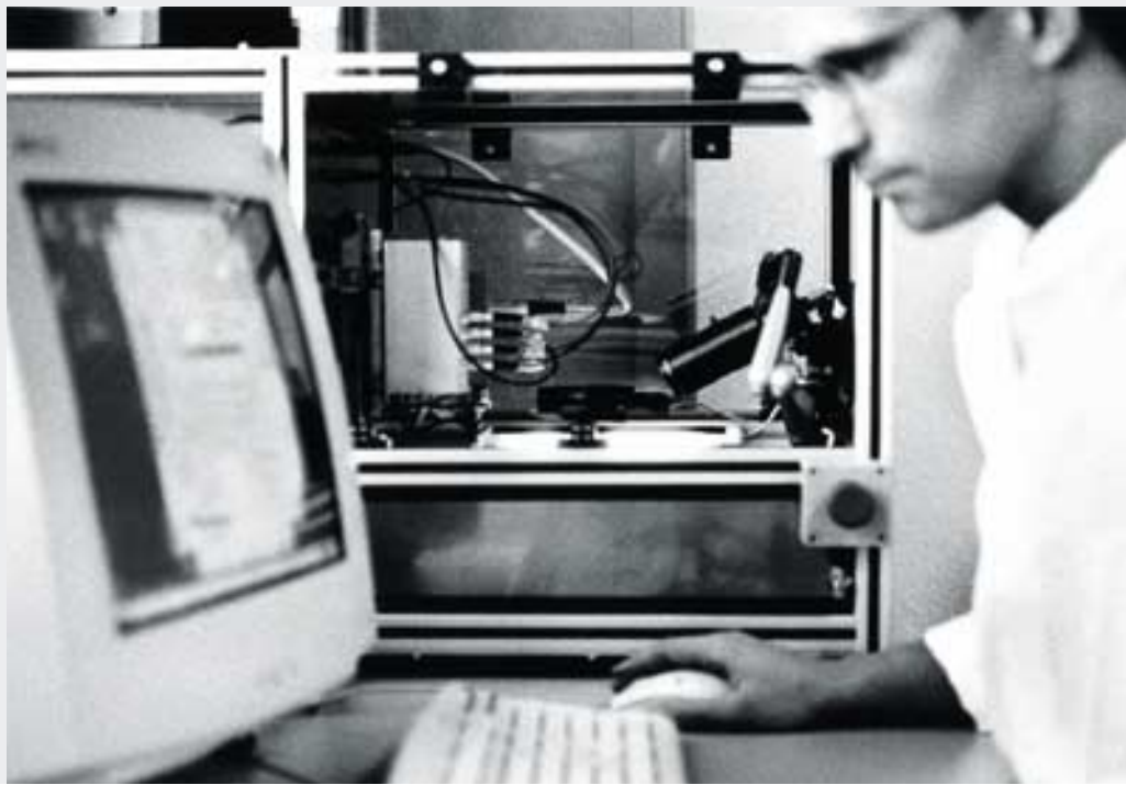
Fig.: Assay systems receive the final check on the MONA and DINA bench-top assay development stations before being transferred to the EVOscreen® unit for high-throughput screening.
